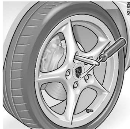
Screwing in assembly aid
